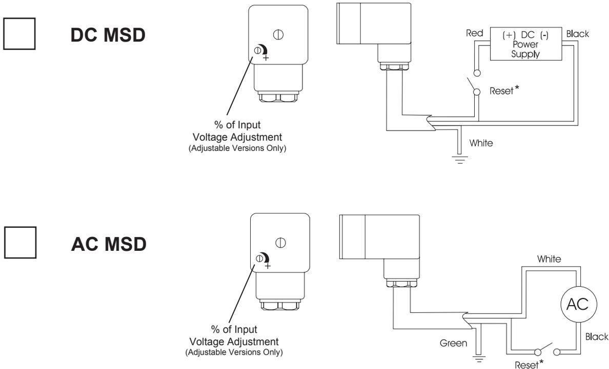
Note: To increase output, turn screw clockwise. To decrease output, turn screw counterclockwise.
